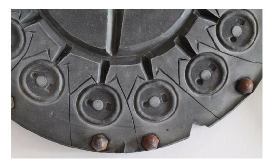
A good example of a correctly gated and vented mould.
